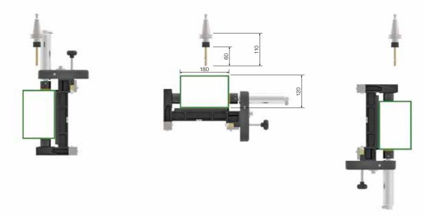
Maximum profile machinable on three surfaces with tool protruding 110 mm from the spindle nose
